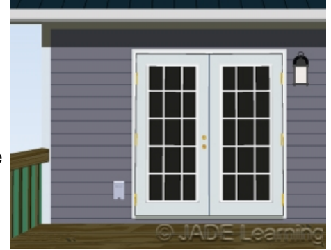
The required outdoor receptacle outlet must be installed at a readily accessible location not more than 6.5 feet above grade level.
