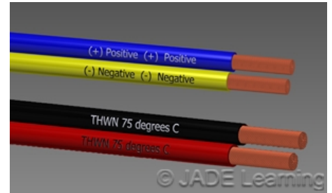
Feeder DC ungrounded conductors of No. 6 AWG or smaller need to be identified by polarity.
