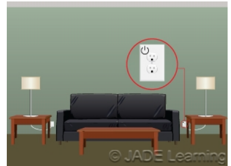
Nonlocking-type 125-volt, 15- and 20-ampere receptacles that are controlled by an automatic control device must be marked with the new symbol.
