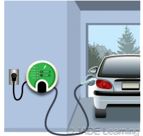
A power-supply cord includes the attachment plug and flexible cord that connects the electric vehicle supply equipment (EVSE) to a receptacle.
