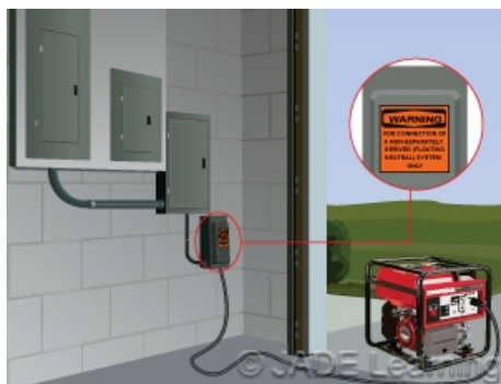
A warning sign is required at the power inlet temporary connection to a portable generator.
