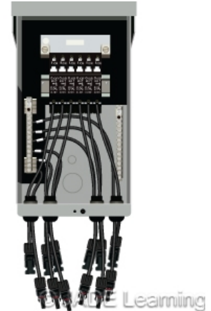
DC combiner disconnects must be in the combiner box or within 6 ft.
